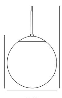
Voltage (V): 230 Volt IP degree: IP20 Maximum bulb wattage (W): 25W Class (Class 1, Class 2, Class 3): Class 2 (Double isolated) Socket type: E27 Dimmerable: Yes with compatible bulb
