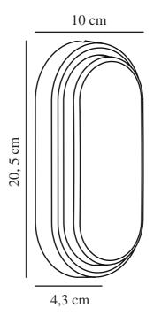
Voltage (V): 230 Volt IP degree: IP54 Class (Class 1, Class 2, Class 3): Class 2 (Double isolated) Socket type: LED Module Parallel connection: True
