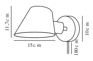
Voltage (V): 220-240 Volt IP degree: IP20
