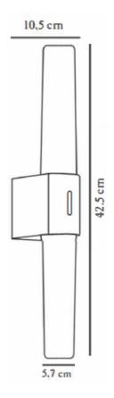
Voltage (V): 230 Volt IP degree: IP44 Class (Class 1, Class 2, Class 3): Class 2 (Double isolated) Socket type: LED Module
