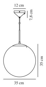
Voltage (V): 230 Volt IP degree: IP20 Maximum bulb wattage (W): 25W Class (Class 1, Class 2, Class 3): Class 2 (Double isolated) Socket type: E27
