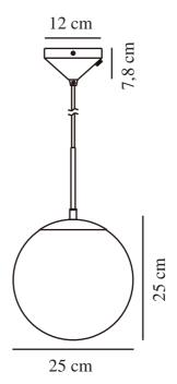
Voltage (V): 230 Volt IP degree: IP20 Maximum bulb wattage (W): 25W Class (Class 1, Class 2, Class 3): Class 2 (Double isolated) Socket type: E27
