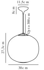
Voltage (V): 220-240 Volt IP degree: IP20 Maximum bulb wattage (W): 40W Class (Class 1, Class 2, Class 3): Class 2 (Double isolated) Socket type: E27
