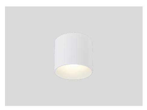
Cylindrical ceiling surface mounted downlight made from die-cast aluminium; surface Signal White; powder coated; matt texture; RAL 9003; optional single inner reflector and single inner cover available; with COB (Chip on Board) technology for maximum efficiency; no appearance of multiple shadows; phase-cut dim; light colour 3000 K; Binning initial 3 MacAdam; CRI 80; 220 - 240 V; degree of protection IP65; PC1; light source replaceable by end-user;
